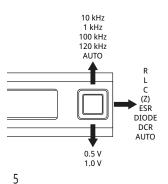
**Note:** To avoid errors do not use the Quick Controls during component measurement. UP – change test ranges DOWN – change test signal levels LEFT/RIGHT – change measurement modes
