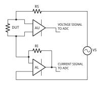
Voltage across the component is generated by the test signal source Vs. Both the amplitude and frequency of Vs can be set. The voltage is applied to the device under test (DUT) through the source resistance Rs. Current flows to the virtual ground of the current amplifier AI, and through the current conversion resistor Ri. The output of AI provides a signal proportional to the current, I\*Ri.
